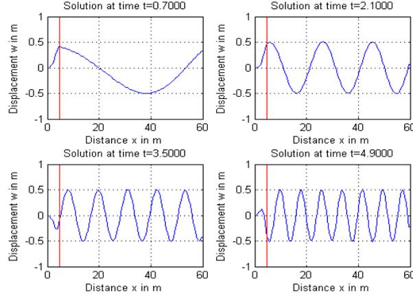
Fig. 1: The optimized feedback controller is applied on the left boundary. A frequency sweep excites the right boundary. No reflections back into the computational domain are visible
