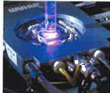
Fig. 2: Electrically contacted high-temperature PV cell (HT-PV) illuminated by 10W LED/365nm
