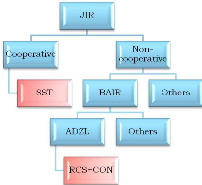
Fig. 3. Overview of Joint Interference Reduction (JIR). SST ... spread-spectrum technology, BAIR ... blind adaptive interference reduction, ADZL ... adaptive dead-zone limiter, RCS ... reliable chip-selector, CON ... threshold control.
