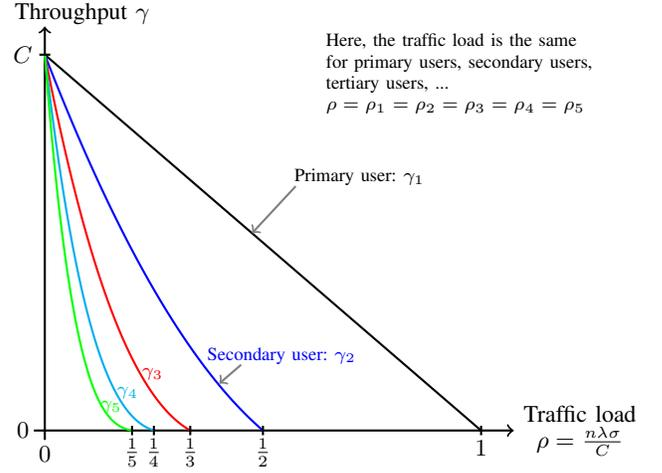
Fig. 2. User throughput for different priority groups. For example, secondary users can access the channel only when no primary user is active, resulting in a lower throughput. If the traffic load is too high, congestion causes the throughput to become zero.
