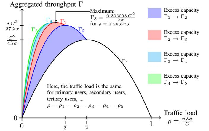
Fig. 3. The aggregated throughput, a measure for social optimality, shows a maximum for a specific traffic load. If there exist only primary users, the maximum aggregated throughput is achieved for a traffic load of  $\frac{1}{2}$ . However, the overall maximum requires at least three priority groups.
