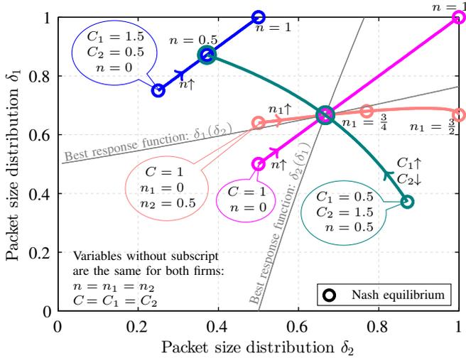
Fig. 5. Best response functions and Nash equilibria for  $\sigma\lambda = 1$  and a few selected values of  $C$  and  $n$ . The Nash equilibrium delivers the throughput maximizing packet size distribution between primary and secondary channel.
