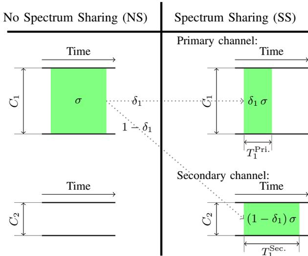
Fig. 4. A packet of size  $\sigma$  is split between primary and secondary channel. Note that throughput maximization requires  $T_1^{\text{Pri.}} = T_1^{\text{Sec.}}$ . Because the required time in the secondary channel depends also on the choices of the other operator, we analyze the outcome using non-cooperative game theory. The Nash equilibrium then corresponds to the optimal load distribution between primary channel and secondary channel.
