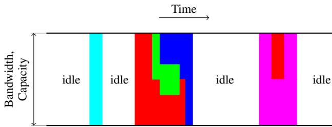
Fig. 1. Dynamic spectrum allocation (statistical multiplexing) means that the capacity is shared (equally) among active users. The instantaneous user throughput then depends on how many users are active and is thus a statistical variable. Note that it can also happen that there are no active users, that is, idle times.
