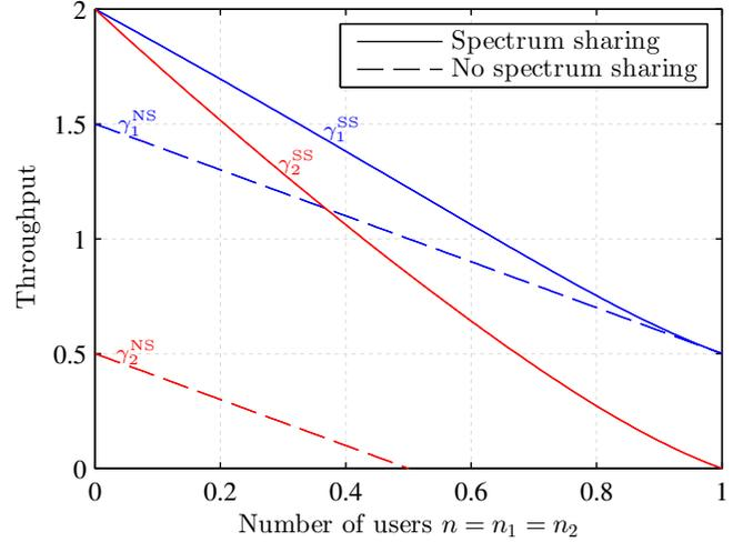
Fig. 6. User throughput in case of no spectrum sharing (NS) and discriminatory spectrum sharing (SS), for the special case of  $C_1 = 1.5$ ,  $C_2 = 0.5$  and  $\lambda\sigma = 1$ . The packet size distribution which maximizes the throughput is shown in Figure 5 (blue curve).
