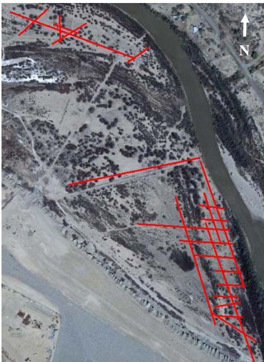
Figure 1. Layout of the TDIP profiles (red lines) collected at the Shiprock site.
