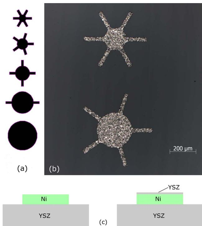
**Figure 1.** (a) Schematic drawing of electrode designs with equal circumference and varying area used in this study. (b) Bright field reflected light microscopic image of typical electrodes after measurement. (c) Schematic side-view of a sample without (lhs) and with a YSZ cover (rhs).
