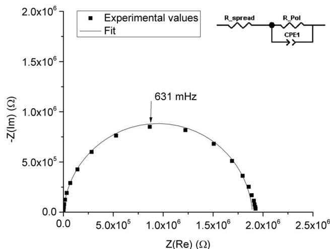
**Figure 2.** Nyquist plot of a typical impedance spectrum (symbols) and corresponding CNLS-fit (line). The equivalent circuit used for fitting is shown in the top right corner. Fit parameters:  $R_{\text{spread}} = 392 \Omega$ ,  $R_{\text{Pol}} = 1.89 \text{ M}\Omega$ ,  $Q_0 = 1.56\text{E-}7 \text{ Ss}^{0.956}$ ,  $n = 0.956$ . Conditions:  $T = 800^\circ\text{C}$ , 2.5% H<sub>2</sub>/0.15% H<sub>2</sub>O/balance Ar, Ni needle.
