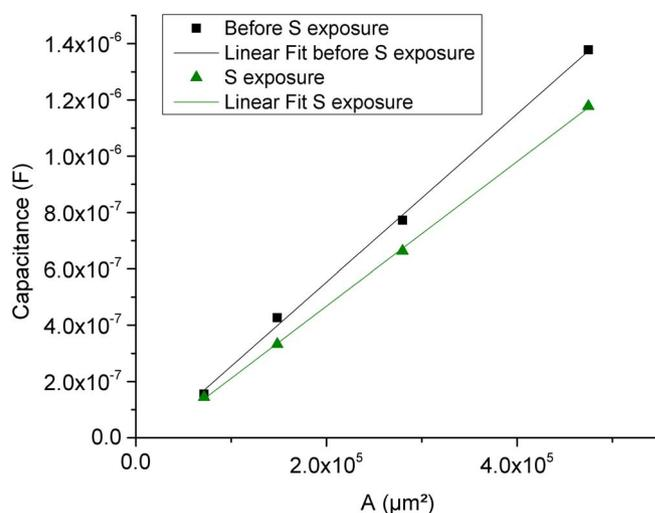
**Figure 5.** Electrode capacitance as a function of electrode area before and during sulfur exposure. The pre-exposure values are from the last measurement before exposure, the sulfur exposed values the last before  $\text{H}_2\text{S}$  removal from the gas feed. Conditions:  $T = 800^{\circ}\text{C}$ , 2.5%  $\text{H}_2/0.15\%$   $\text{H}_2\text{O}/(10 \text{ ppm } \text{H}_2\text{S})/\text{balance Ar}$ , Ni needle.
