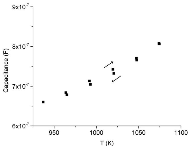
**Figure 8.** Temperature dependence of the electrode capacitance. The measurement was performed on an electrode with an area of 0.280 mm<sup>2</sup> by first decreasing and then increasing the temperature. Conditions:  $T = \text{var.}^{\circ}\text{C}$ , 2.5% H<sub>2</sub>/0.15% H<sub>2</sub>O/balance Ar, Ni needle.
