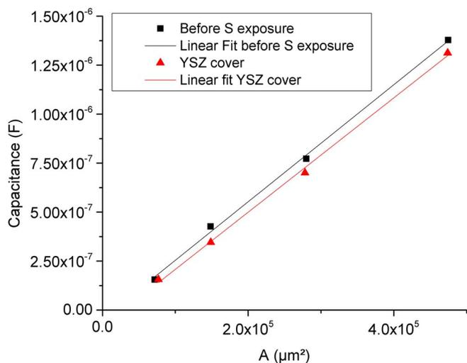
**Figure 6.** Comparison of capacitance values of electrodes with and without a YSZ cover on top of the Ni. Values for uncovered electrodes were taken from electrodes before sulfur poisoning (see Figure 5). Conditions:  $T = 800^\circ\text{C}$ , 2.5%  $\text{H}_2/0.15\%$   $\text{H}_2\text{O}/\text{balance Ar}$ , Ni needle.
