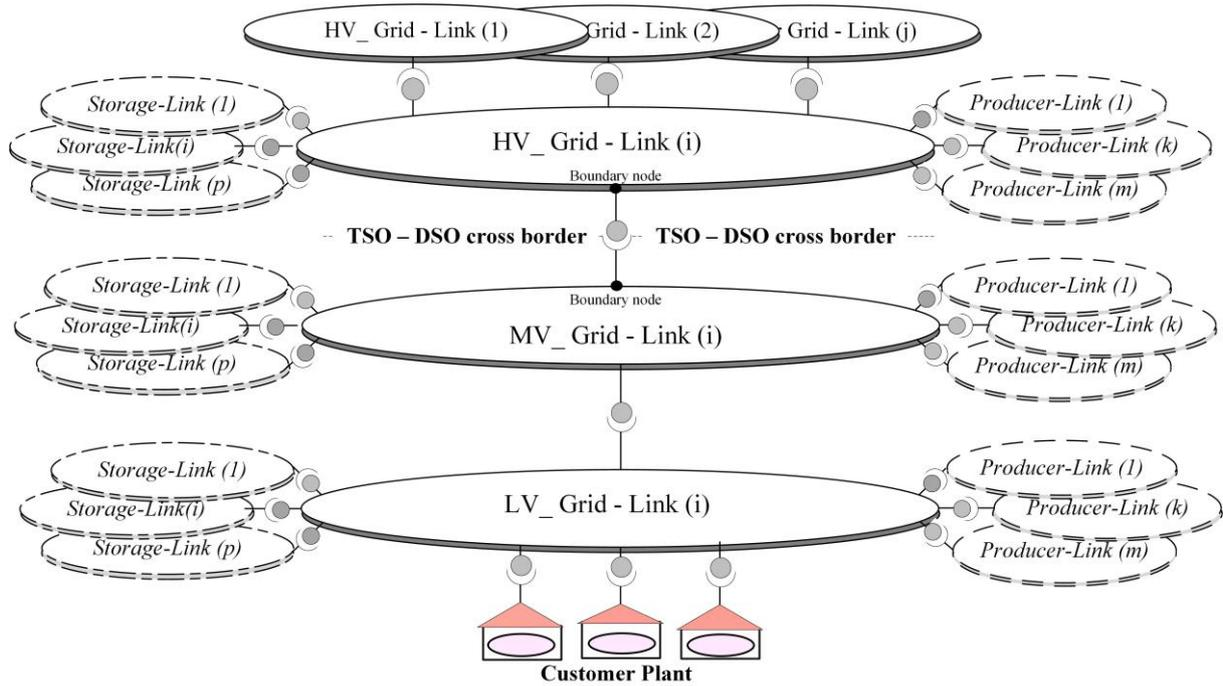
Fig. 3 *LINK* – based technical/functional architecture of power systems in the new electricity era.
