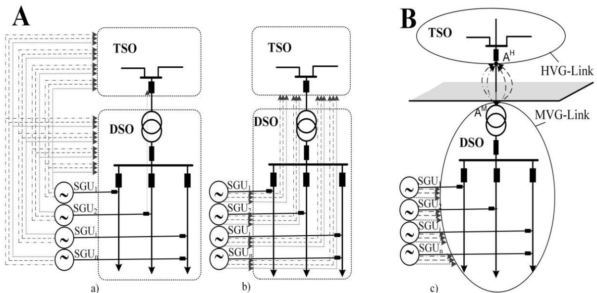
Fig. 5 Data flow from DSO to TSO: a) demand facilities communicates directly to its TSO and DSO; b) demand facilities communicates via its DSO to the TSO; c) data exchange in the case of *LINK*-based architecture.
