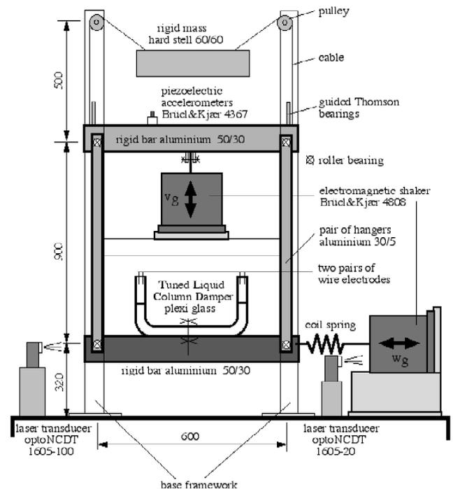
Figure 1: Small-scale testing facility
