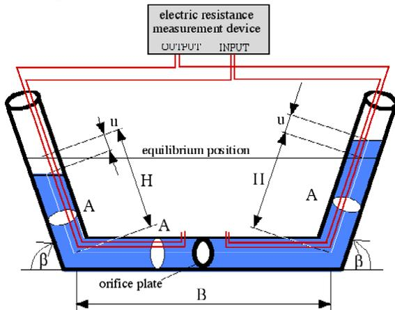
Figure 2: TLCDC with moving liquid mass
