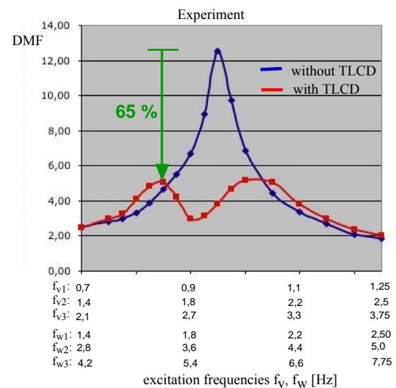
**Fig. 2:** Experimentally obtained DMF, horizontal displacement of the bridge
