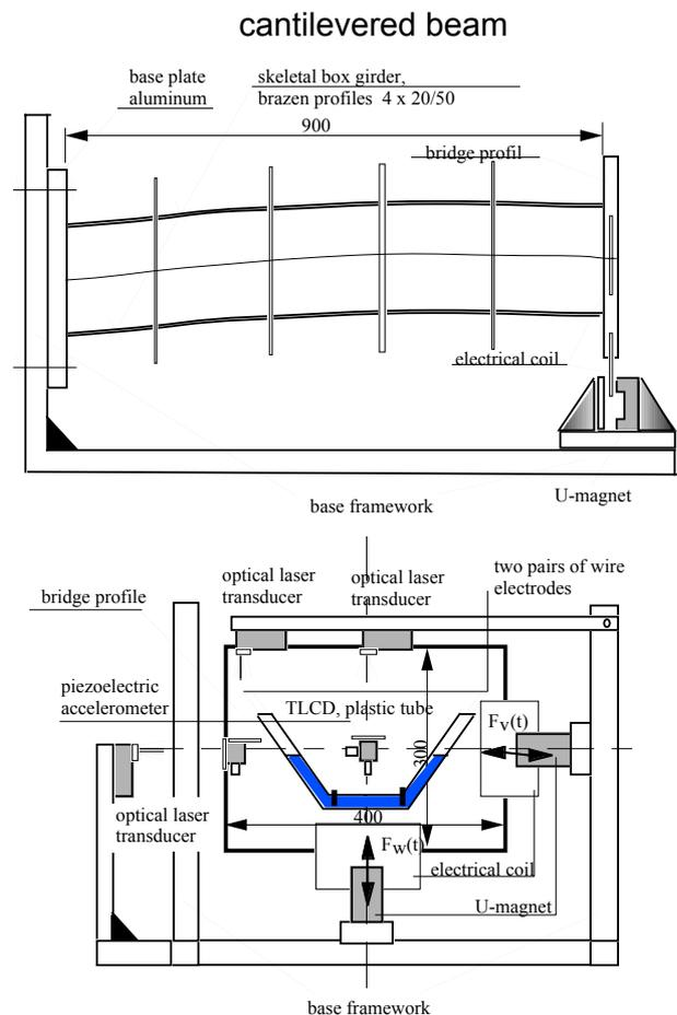
**Fig. 1:** Side and front view of the constructed three DOF bridge model with attached TLCD
