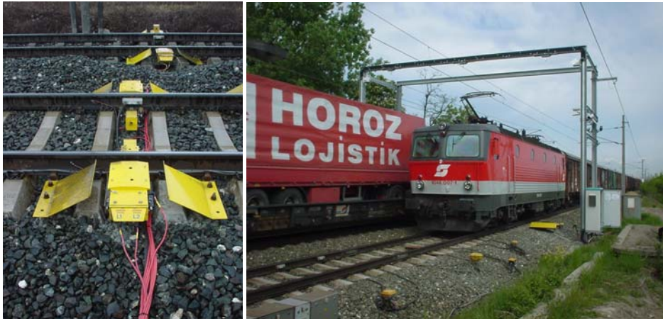
Figure 4 (left): Hot box detection system at the Checkpoint prototype. Manufacturer: ÖBB Infrastruktur Betrieb AG, Vienna (Austria). Figure 5 (right): Train gauge monitoring system at the Checkpoint prototype. Manufacturer: ASE Industry Services AG, Bruchsal (Germany), on behalf of ÖBB infrastructure Bau AG, Vienna (Austria).
