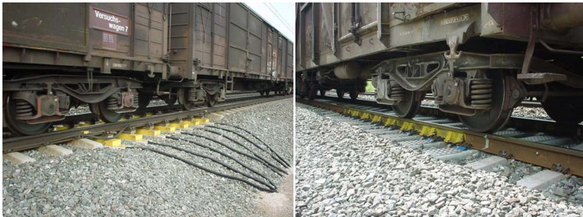
Figure 2 (left): Dynamic scale at the Checkpoint prototype. Manufacturer: SCHENCK PROCESS GmbH, Darmstadt (Germany).
