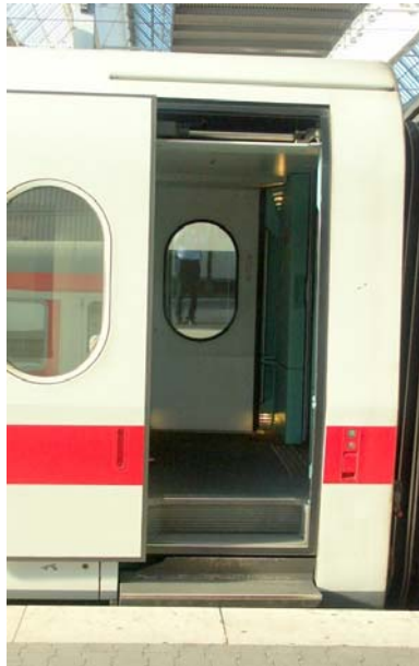
Fig. 4: Favourable entrance situation; 2 steps, 90 cm door width, gentler gradient in the angle of the steps.
