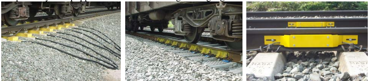
Figure 1 (left): Dynamic scale at the Checkpoint prototype. Manufacturer: SCHENCK PROCESS GmbH, Darmstadt (Germany).
