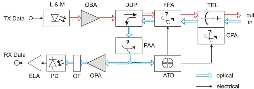
Fig. 1. Basic block diagram of an optical transceiver for space-to-space links (L & M..laser and modulator, OBA..optical booster amplifier, DUP..optical duplexer, FPA..fine pointing assembly, TEL..telescope (optical antenna), CPA..coarse pointing assembly, PAA..point ahead assembly, ATD..acquisition and tracking detector, OPA..optical pre-amplifier, OF..optical bandpass filter, PD..photo detector, ELA..electronic amplification and data recovery).
