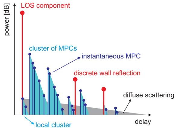
Figure 2: Illustration of model components in the delay domain: LOS, discrete reflections, clusters, MPCs, and diffuse scattering.
