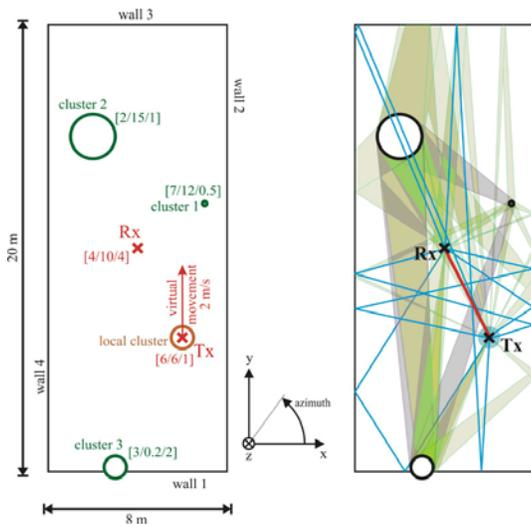
Figure 3: Room layout with physical clusters and link ends, and considered propagation paths.
