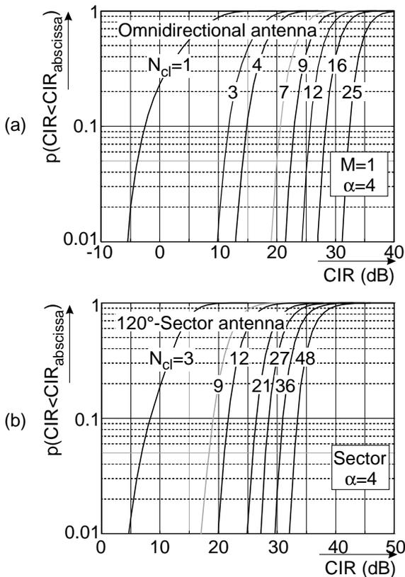
Fig. 1: CDF of the CIR,  $p(\text{CIR} < \text{CIR}_{\text{abcissa}})$ , i.e. the outage probability  $P_{\text{out}}$ , for (a): a system using omnidirectional antennas, and (b): a system using  $120^\circ$ -sector antennas, with the cluster size  $N_{cl}$  as parameter. The curves are read in the following way: (a) For a cluster size of  $N_{cl} = 7$  the CIR is less than or equal to 20dB in  $P_{\text{out}} = 5\%$  of the cases.
