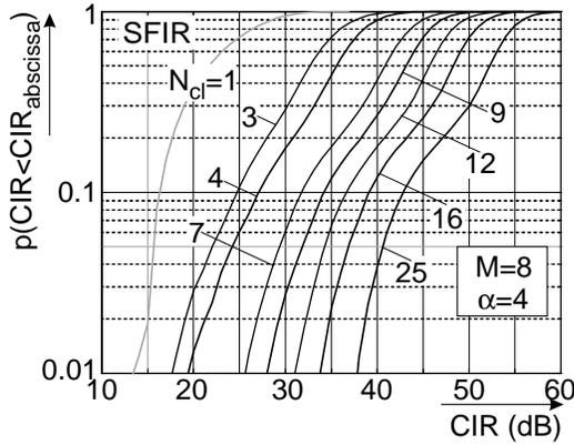
Fig. 3: CDF of the CIR,  $p(\text{CIR} < \text{CIR}_{\text{abcissa}})$ , i.e. the outage probability  $P_{\text{out}}$ , for a system using three or four ULAs with  $M = 8$  at one cell site with the cluster size  $N_{cl}$  as parameter.
