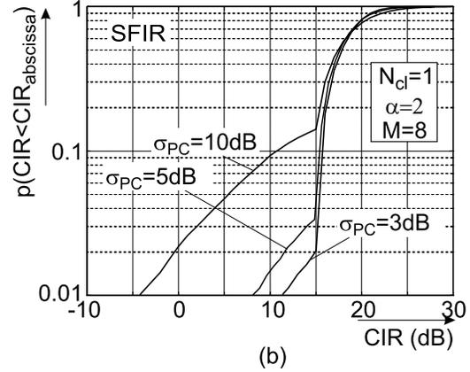
Fig. 4: Influence of power control errors on the CIR. CDF of the CIR,  $p(\text{CIR} < \text{CIR}_{\text{abcissa}})$ , i.e. the outage probability  $P_{\text{out}}$ , versus the CIR for an SFIR–system with  $N_{cl} = 1$ ,  $M = 8$  with the standard deviation of the power control error,  $\sigma_{PC}$ , as parameter. (a)  $\alpha = 4$ , (b)  $\alpha = 2$ .
