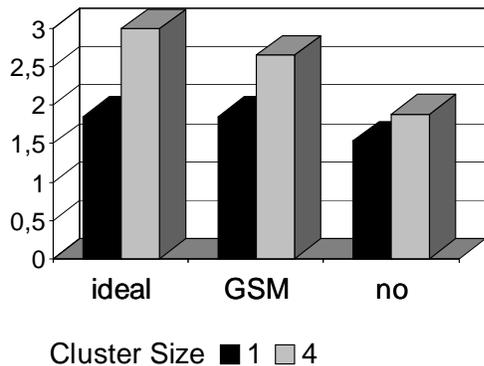
Fig. 7: Mean number of users for ideal, GSM, and no power control for different cluster sizes.
