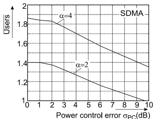
Fig. 6: Influence of power control errors with standard deviation  $\sigma_{PC}$  on the mean number of users.
