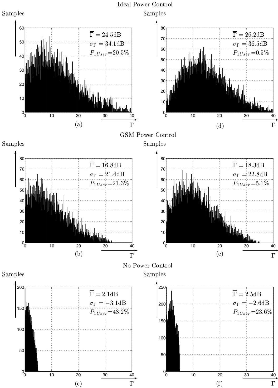
Fig. 8: Distribution of  $\Gamma$ . (a) – (c) for cluster size  $N_{cl} = 1$ , (d) – (f) for cluster size  $N_{cl} = 4$  with ideal, GSM, and without power control, respectively.  $P_{1User}$  is the probability that only one user is accepted in the center cell.
