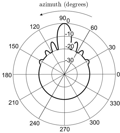
Fig. 2: Antenna pattern of an eight–element ULA with spacing  $d = 0.5\lambda$ , and null depth and front–to–back ratio of 20dB.
