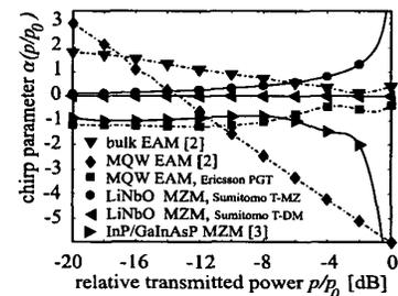
**CThL50** Fig. 1. Chirp parameter  $\alpha$  as function of transmitted power for different electroabsorption and Mach-Zehnder modulator types (own measurements and<sup>2,3</sup>).
