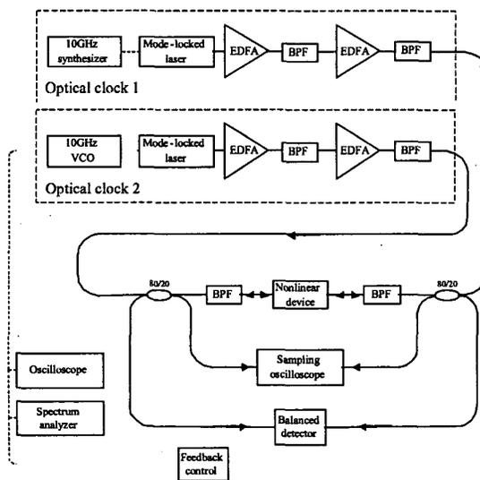
**CThL51** Fig. 1. Schematic diagram of bi-directional nonlinear timing system for clock locking. Solid lines indicate optical connections, while dashed lines represent electrical connections.
