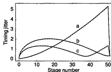
**CThL49** Fig. 1 Timing jitter (ps) plotted as a function of stage number for the parameters described in the text. (a) No pre-compensation and complete post-compensation. (b) Complete pre-compensation and no post-compensation. (c) Optimal combination of pre- and post-compensation.
