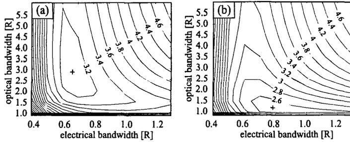
**CThL50** Fig. 2. Receiver sensitivity penalty [dB] relative to the quantum limit as function of both electrical and optical bandwidth (normalized to data rate R) for (a) chirp-free NRZ transmission and for (b) chirped NRZ signals using modulator type “p” of Fig. 1.
