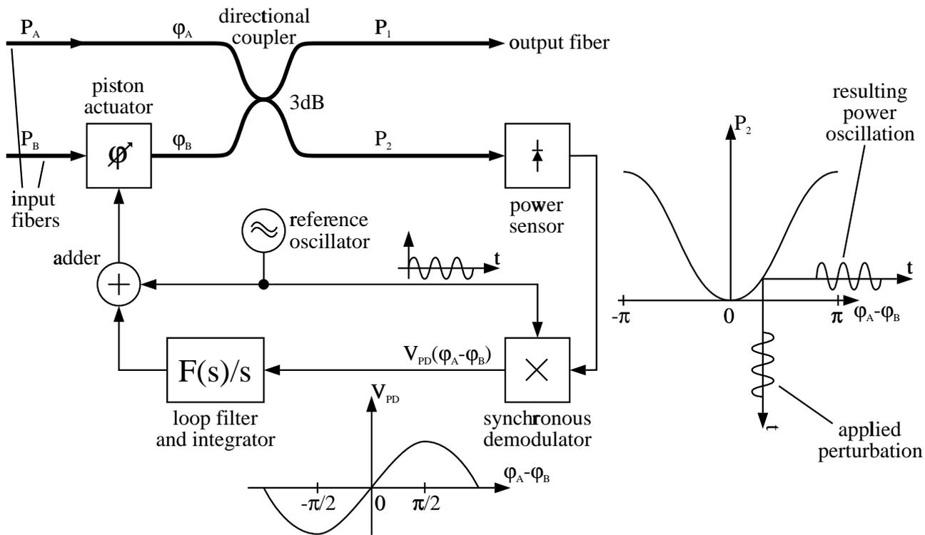
Fig. 3: An optical phase-locked loop employing a sinusoidal perturbation for piston sensing
