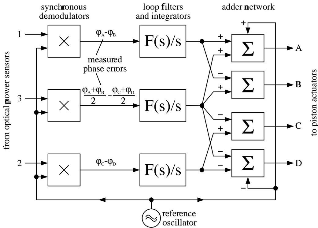
Fig. 4: Block diagram of the piston control unit
