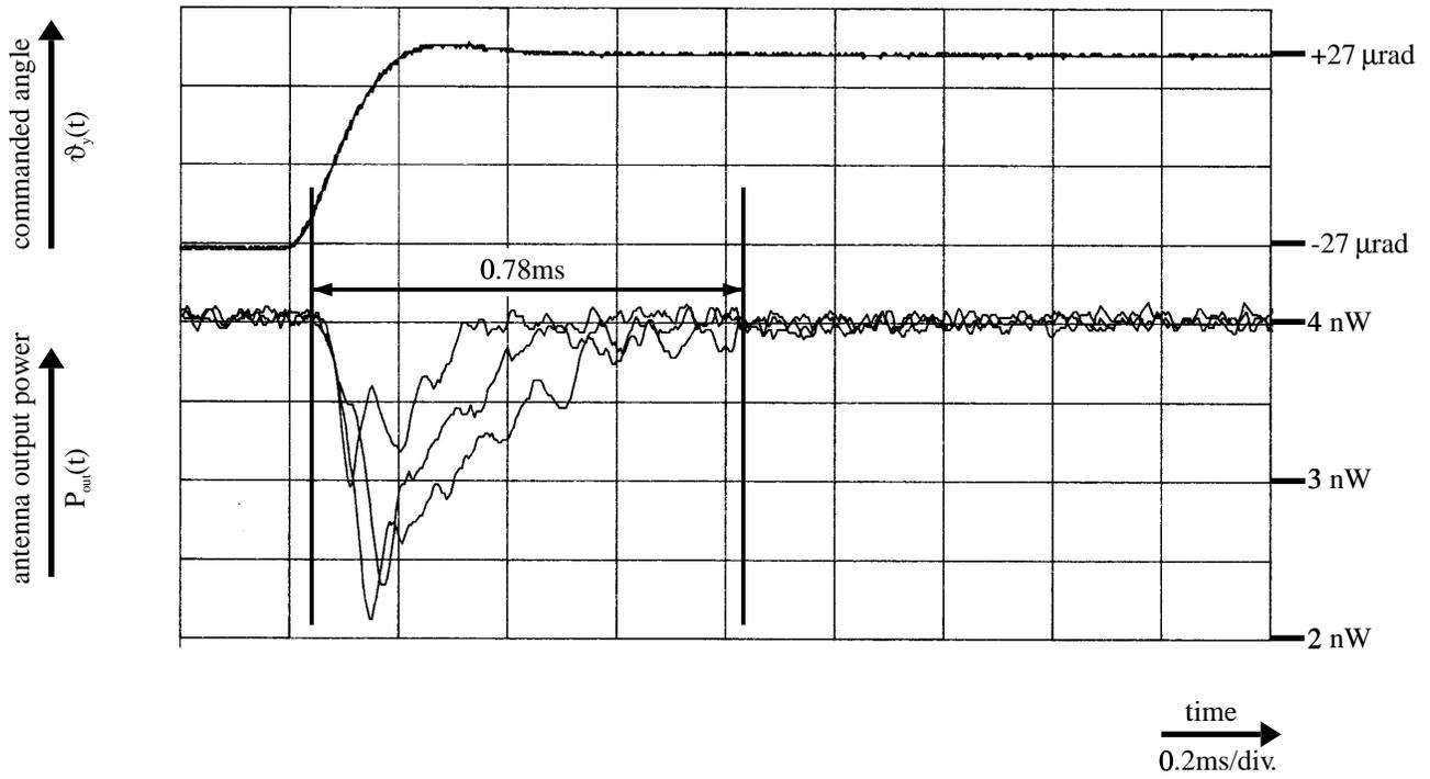
Fig. 7: Measured response to a step-shaped change of the input wave direction. The occurrence of different traces is referred to in the text. The response time amounts to 0.78ms.
