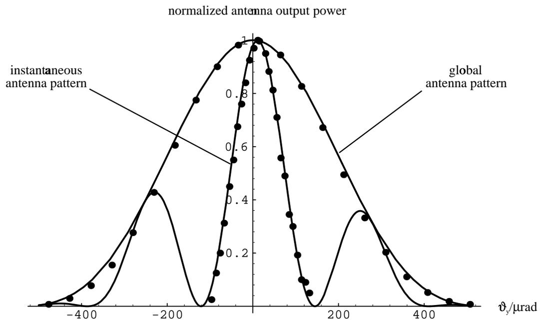
Fig. 6: Global antenna pattern and instantaneous antenna pattern (dots ... measured, solid lines ... calculated)
