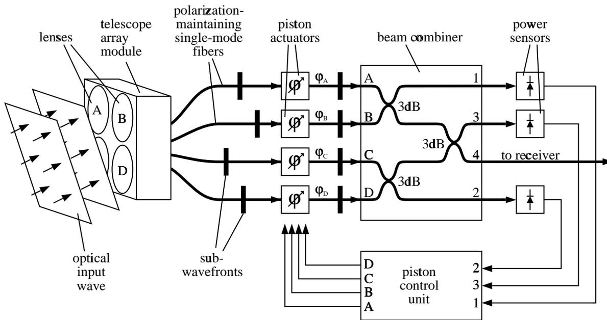
Fig. 1: Block diagram of the experimental four-aperture receive antenna
