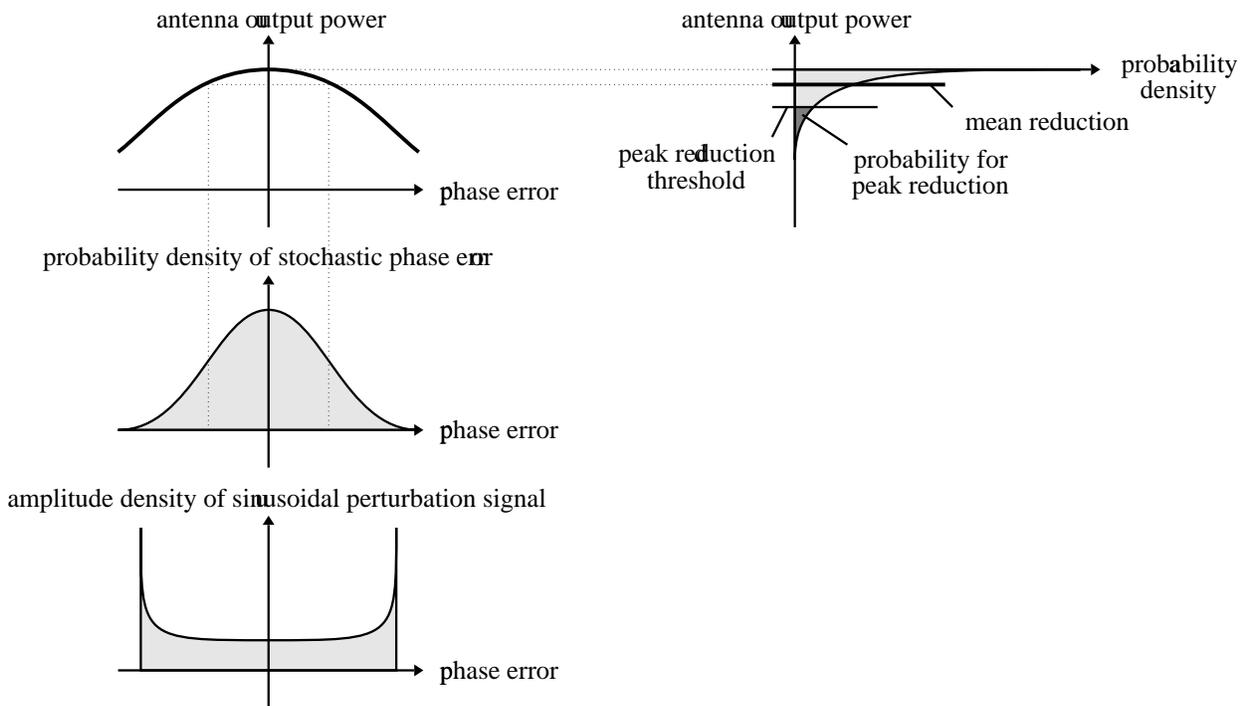
Fig. 8: Influence of the residual phase error on the distribution of the antenna output power
