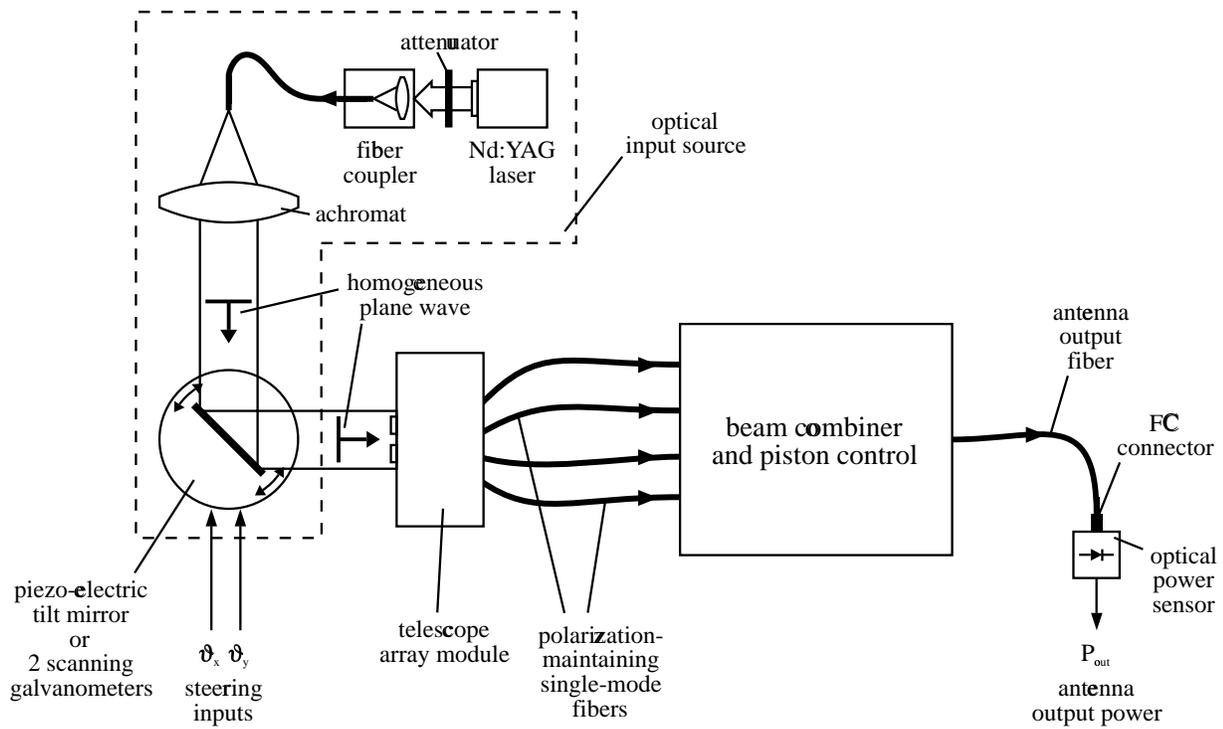
Fig. 5: Basic test setup
