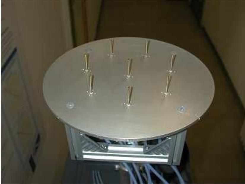
**Figure 5.5:** The 7 + 1 omnidirectional uniform circular monopole Tx array.
