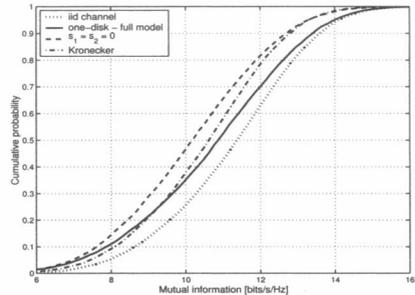
Fig. 2. Mutual information CDF for two correlation models based on the one-disk model (MIMO  $2 \times 2$ , SNR = 20 dB; element spacing:  $0.28 \lambda$ )
