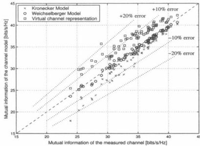
Fig. 1. Mutual information of three analytical models vs. measured values (MIMO  $8 \times 8$ , SNR = 20 dB)
