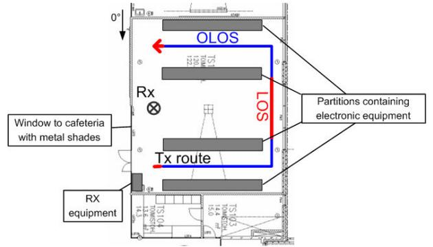
Figure 2. Measurement route in the medium-sized laboratory; Antenna orientation for  $0^\circ$  is the same for both Rx and Tx.
