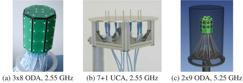
Figure 1. Antenna arrays. (a) 2.55 GHz omni-directional patch array, (b) 2.55 GHz circular monopole array, (c) 5.25 GHz omni-directional patch array.
