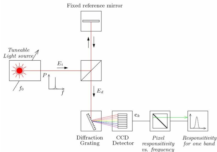
**Figure 2. Measurement setup. for characterizing our spectral encoded FD-OCT with a wavelength swept lightsource. The tuneable light source used for characterization (Superlum Broadlighter 840) delivered a spectral tuning range of more than 50 nm @ 5mW and had a spectral linewidth of less than 0.04 nm.**
