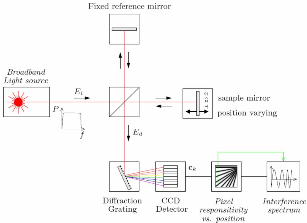
**Figure 3. Setup for mirror measurement; the mirror was manually positioned to obtain reflectivity profiles from different positions within the depth-range.**
