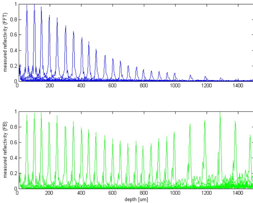
**Figure 4. Mirror results –reconstructed reflectivities (upper blue: FT-based processing, lower green: FB-based processing).**
