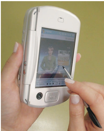
Figure 1. Test equipment: VPA IV UMTS/WLAN
