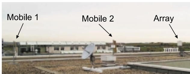
Figure 2: Measurement setup on the roof top of the Alcatel building. The two mobiles are angularly separated by 19^\circ and have a LOS to the base station array.
