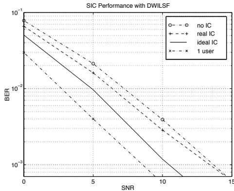
Fig. 5. Performance of DWLSF with serial interference cancellation (SIC)
