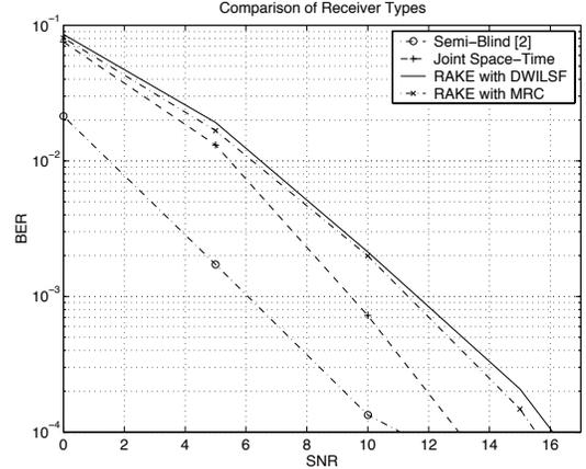
Fig. 3. Comparison of studied receiver types, SDMA scenario
