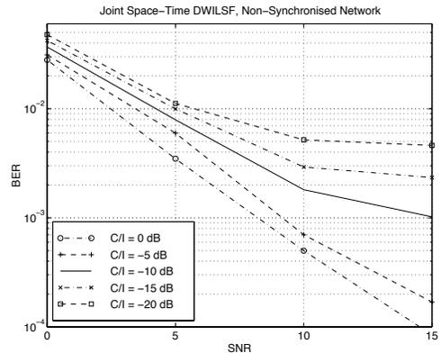
Fig. 4. Performance of Joint Space-Time DWILSF, non-synchronised SFIR scenario
