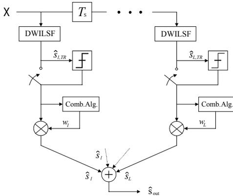
Fig. 1. Principle of the DWILSF-RAKE Receiver
