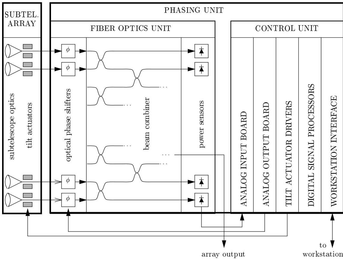
**Figure 2.** Block diagram of the 16 aperture engineering demonstrator
