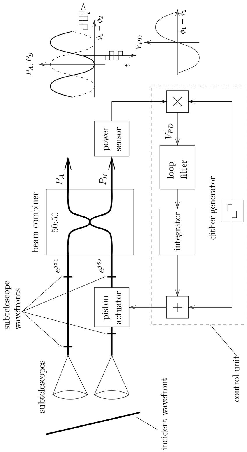
**Figure 1.** Basic principle of the piston control loop employed in the phased array demonstrator
