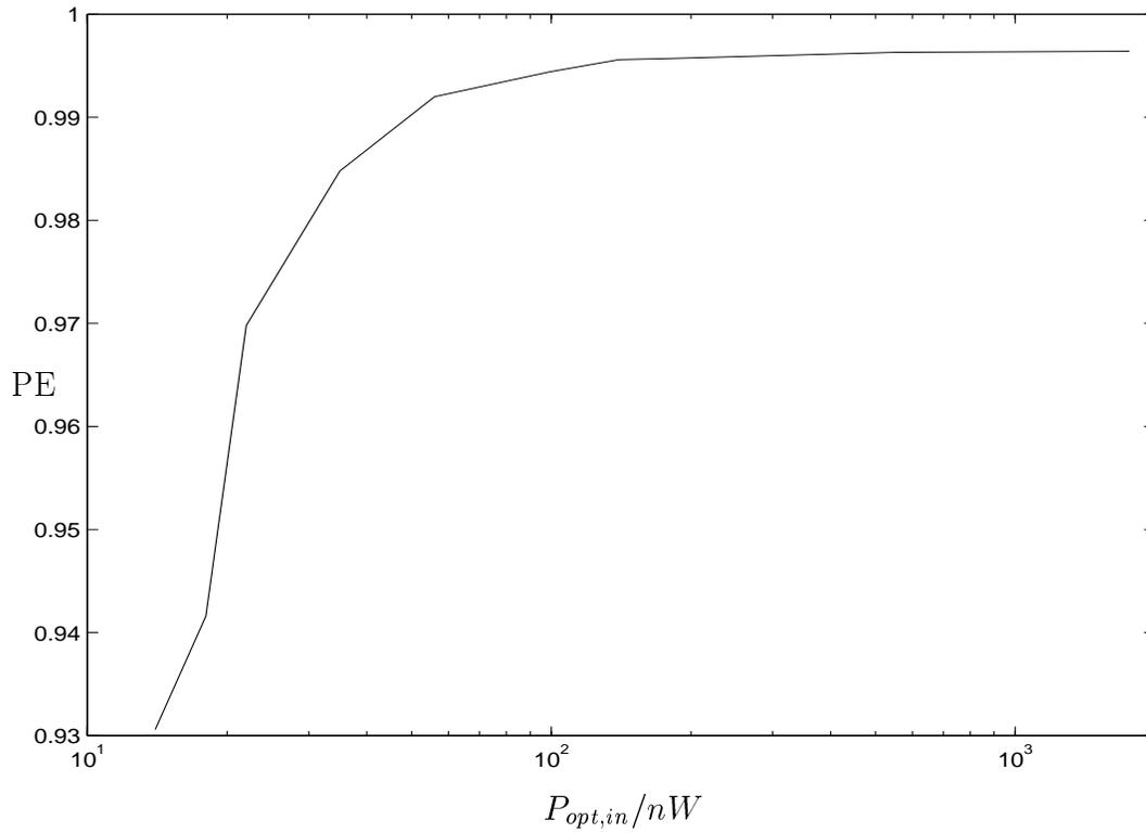
**Figure 7.** Phasing efficiency as a function of total incident power
