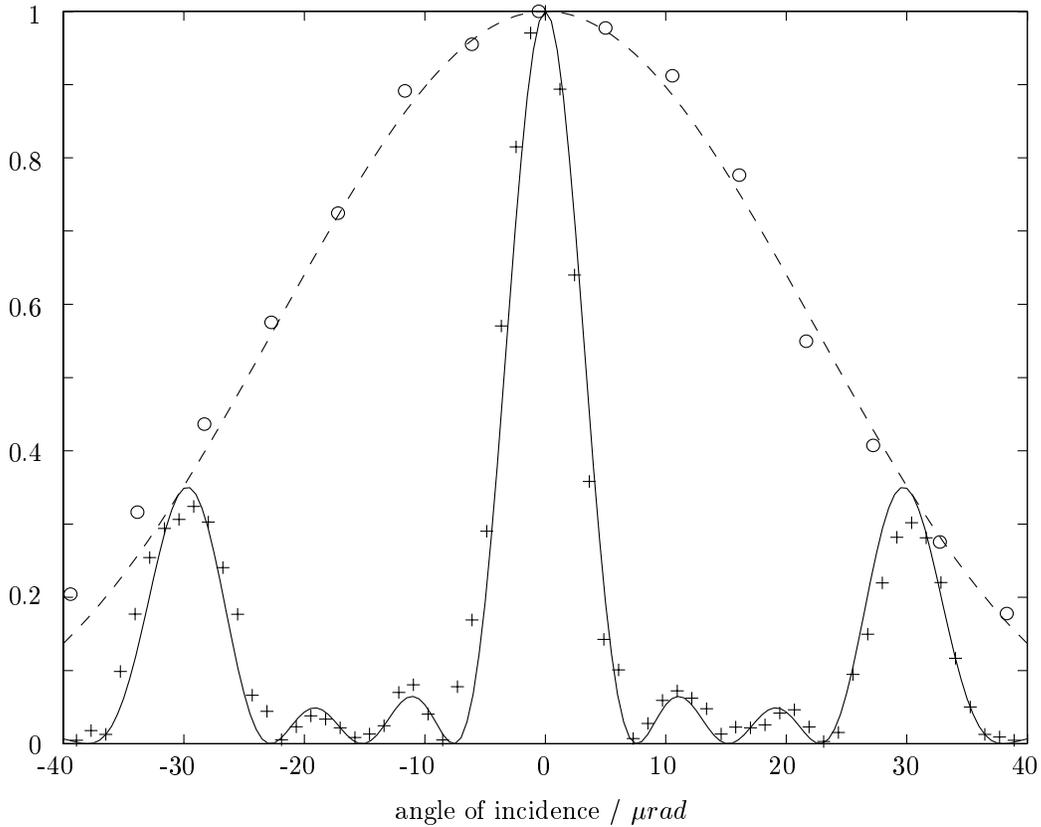
**Figure 5.** Vertical cross section of the receive characteristic (dashed line ... theory; circles ... measurement), and of the instantaneous array characteristic (solid line ... theory; crosses ... measurement)
