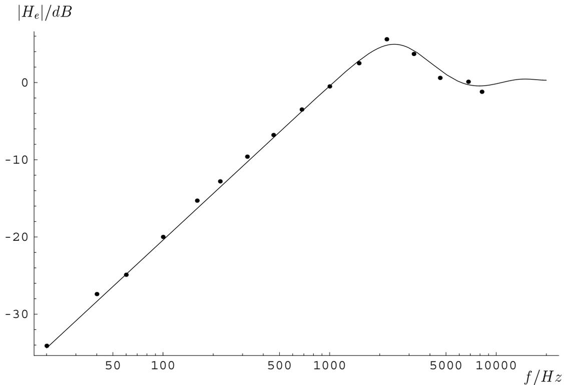
**Figure 6.** Calculated (solid line) and measured (dots) tracking error response of the phased array demonstrator
