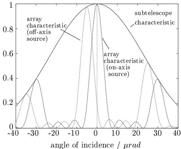
Figure 4: Cross-section of the normalized subtelescope characteristic and of the normalized array characteristic
