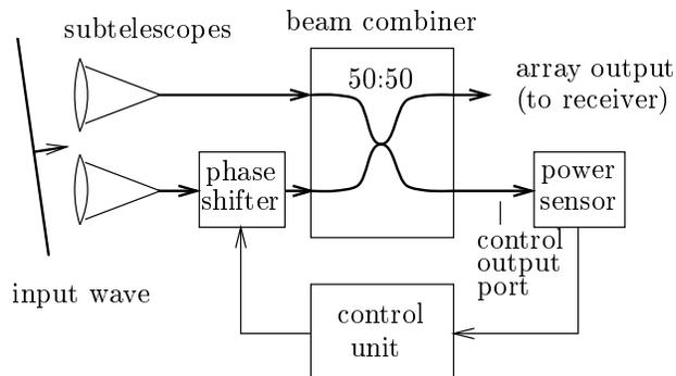
Figure 1: Basic concept of the phased telescope array
