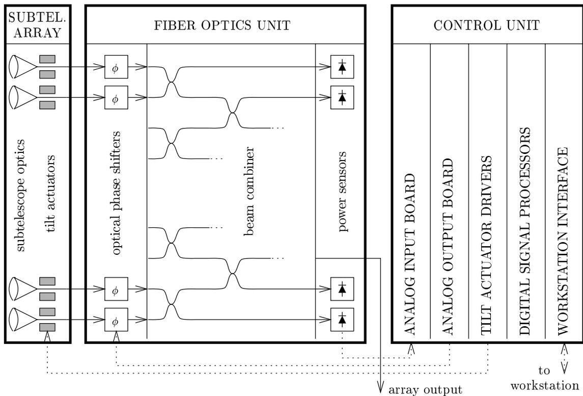
Figure 3: Block diagram of the 16 aperture engineering demonstrator
