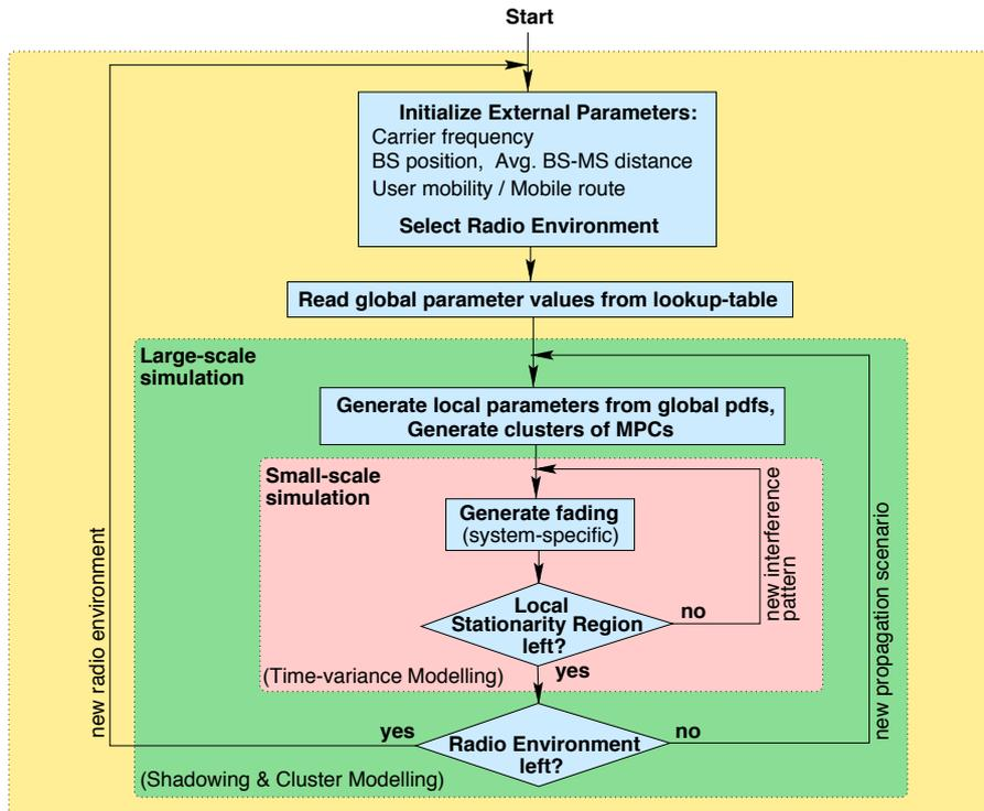
Figure 1: Application of the COST259 SWG2.1 directional channel model.
