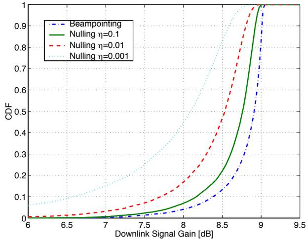
**Figure 3: Downlink signal gain as a function of the diagonal loading factor (AS=5°).**
