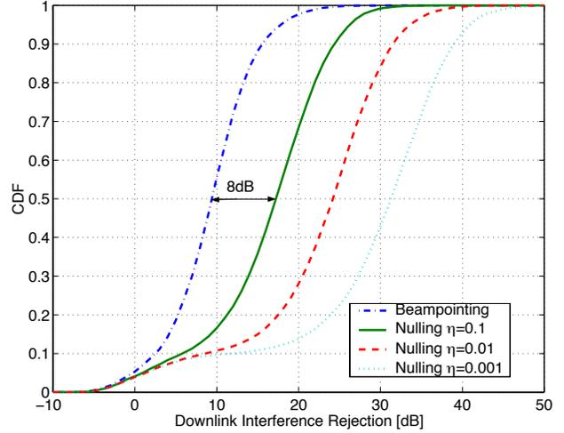
**Figure 4: Downlink interference rejection - 10% packet and 90% circuit switched users (AS=5°).**
