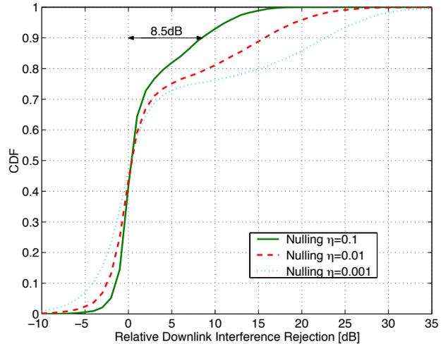
**Figure 5: Relative downlink interference rejection - 75% packet switched and 25% circuit switched users (AS=5°).**
