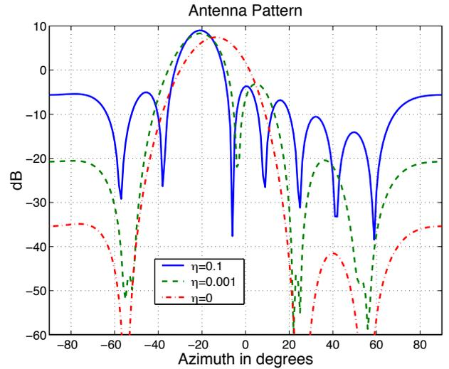
**Figure 1: Antenna pattern with different diagonal loading factors and therefore varying null depth.**
