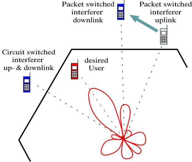
**Figure 2: Change in the traffic channel allocation from uplink to downlink. The arrow denotes the change of packet switched traffic allocation from up- to downlink.**
