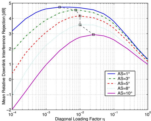
**Figure 7: Mean relative downlink interference rejection - 75% packet switched and 25% circuit switched users.**
