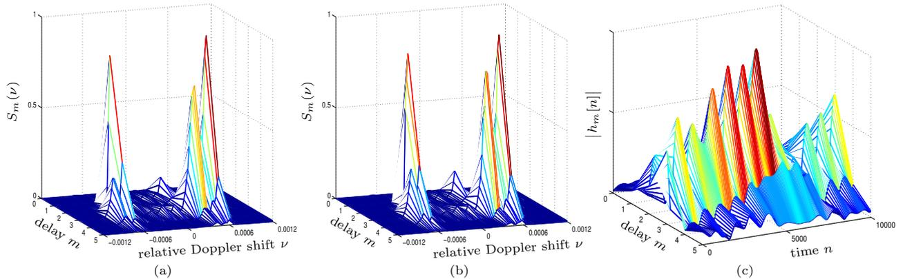
**Figure 4:** Simulation of a realistic channel: (a) Specified scattering function (estimated from measured channel data); (b) simulated scattering function (estimated from realizations of the simulated impulse response); (c) magnitude of a realization of the simulated impulse response.
