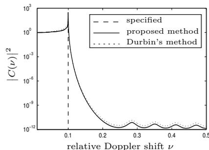
**Figure 3:** Squared magnitude of the frequency responses of the subsampled ARMA filter obtained with the proposed MA design method and with Durbin's method.
