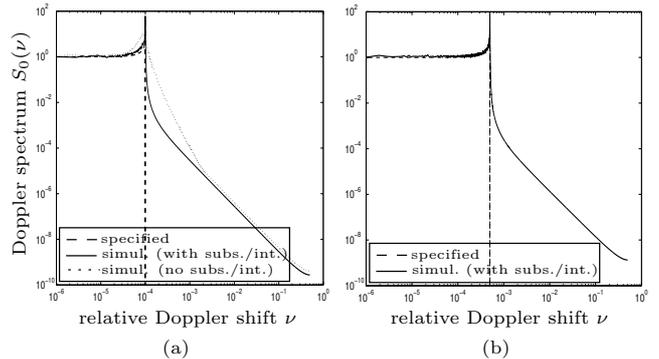
**Figure 2:** Simulation of a single-tap channel: (a) Specified (Jakes) Doppler spectrum, simulated Doppler spectrum, and simulated Doppler spectrum obtained without subsampling/interpolation; (b) simulated Doppler spectrum obtained at the output of the second interpolator stage.
