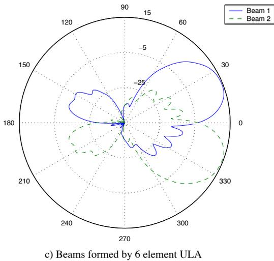
Fig. 3. Antenna pattern of sector antenna (a), beam patterns formed by 4 element ULA (b) and 6 element ULA (c). Radial unit is dBi.
