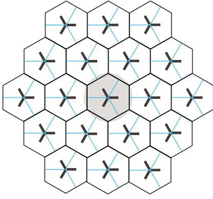
Fig. 2. Simulation area with 19 3-sectored base station sites
