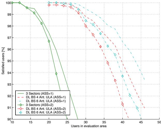
Fig. 4. Percentage of satisfied users versus number of users in the center area for the reference system using sector antennas (solid line), a system using downlink beam switching with 4-element ULAs (dashed line) and a system using downlink beam switching with 6-element ULAs (dash dotted line). The curves for systems allowing a maximum active set size of two have diamond markers where systems not allowing SHO ( $max\_ass=1$ ) have no markers.
