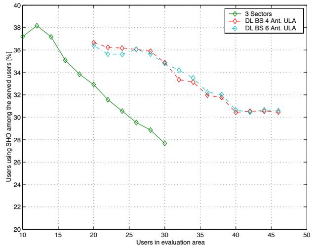
Fig. 5. Percentage of served users using SHO for 3-sector antenna (solid line), downlink beam switching with 4-element ULA (dashed line) and 6-element ULA (dashed dotted line).
