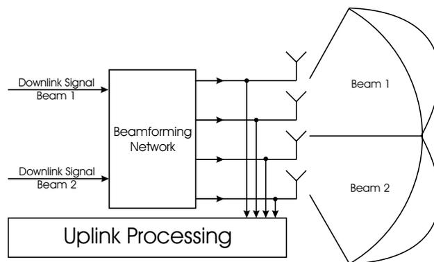
Fig. 1. Principal of downlink beam switching
