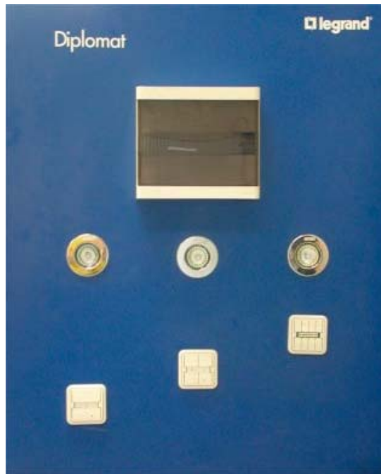
Figure 2: EIB installation used for testing
