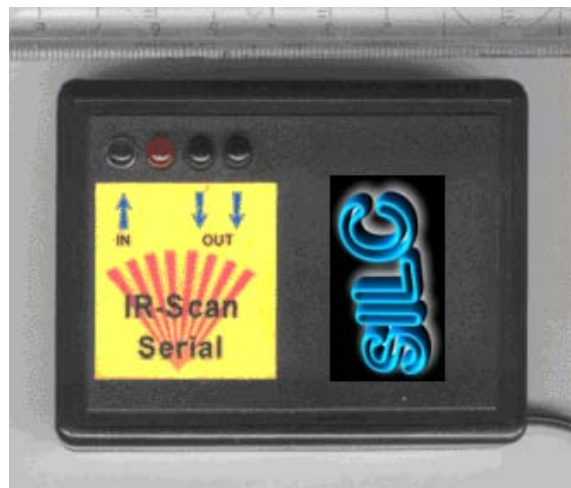
Figure 1: Infrared receive/transmit box for serial port (Producer: Meschik and Partner KEG [5])
