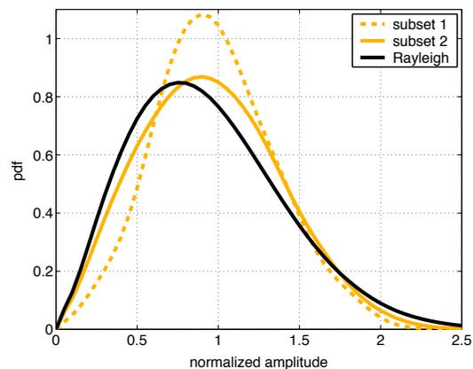
**Fig. 5.** PDF of measured envelope amplitudes in comparison with the Rayleigh distribution. The measured data was divided into two distinct subsets yielding two statistical ensembles.
