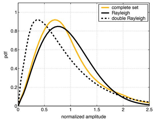
**Fig. 4.** PDF of measured envelope amplitudes in comparison with the Rayleigh and double-Rayleigh distributions. The statistical ensemble comprises the entire measurement set.
