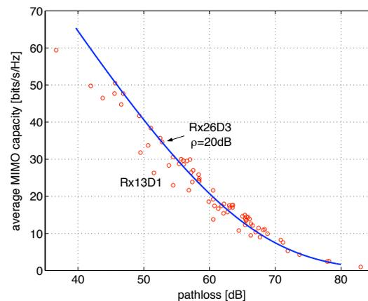
**Fig. 3.** MIMO capacity for different scenarios in an indoor office environment vs. pathloss
