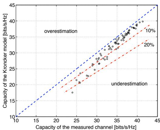
**Fig. 2.** Scatter plot of average ‘Kronecker’ model capacity vs. average capacity of measured channel for an  $8 \times 8$  MIMO system
