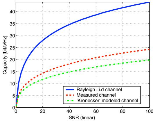
**Fig. 1.** Estimated capacity for Rayleigh i.i.d, measured and synthesized channel, RX position Rx13, direction D1
