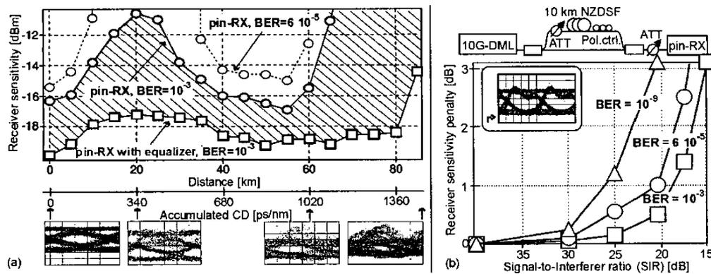
Fig. 3 : (a) Receiver sensitivity (solid:  $BER=10^{-3}$ , dashed:  $BER=6 \cdot 10^{-5}$ ) vs. transmission distance for the 1550-nm CWDM laser. Circles: Unequalized receiver. Squares: Equalized receiver. Hatched area: Equalization gain. Optical eye diagrams shown at various distances. (b) Sensitivity penalty for the unequalized receiver and the 1550-nm channel vs. SIR at  $BER = 10^{-9}$ ,  $6 \cdot 10^{-5}$ , and  $10^{-3}$ .
