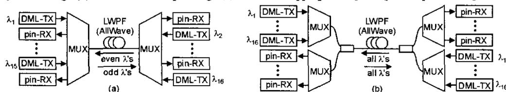
Fig. 1 : (a) 16-channel CWDM system: 8 channels East, 8 channels West. (b) 32-channel CWDM system: 16 channels each direction.
