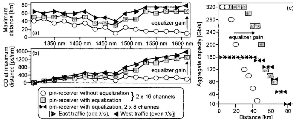
Fig. 4 : (a): Maximum transmission distance for all CWDM channels. (b): Accumulated chromatic dispersion (CD) at maximum distance for each channel. (c): Total system capacity as a function of distance.
