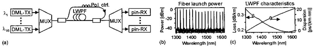
Fig. 2 : (a): Experimental setup for bidirectional CWDM transmission. (b): CWDM spectrum launched bidirectionally into fiber. (c): Loss and dispersion of LWPF.
