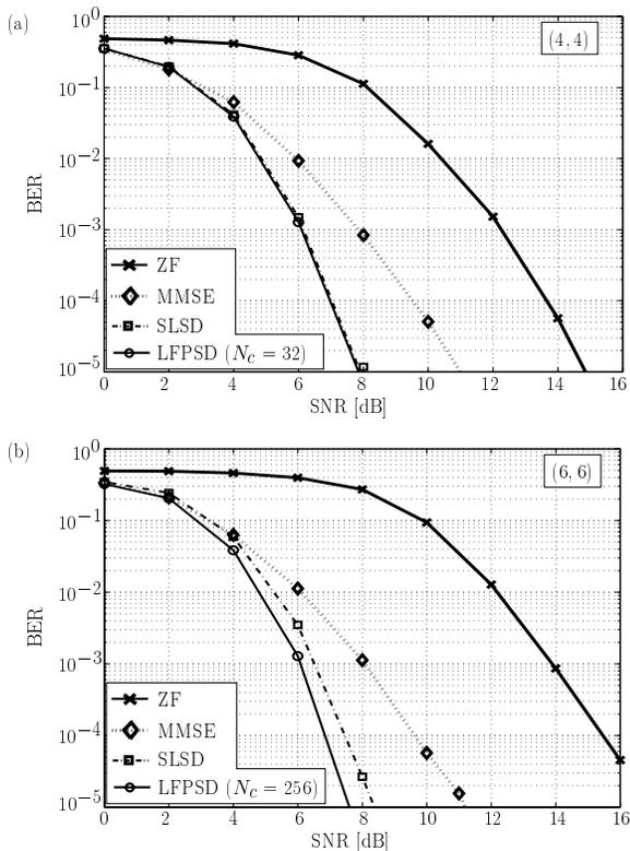
Fig. 4. BER performance of the proposed SLSD, the ZF-based and MMSE-based demodulators, and the LFPSD demodulator for 4-QAM (QPSK) modulation: (a) (4, 4) channel, (b) (6, 6) channel.
