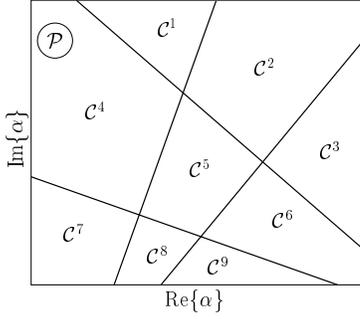
Fig. 2. Cell partitioning of the real reference plane  $\mathcal{P}$  for a (2, 2) MIMO system and 4-QAM modulation.
