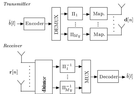
Fig. 1. Block diagram of a MIMO-BICM system [3].
