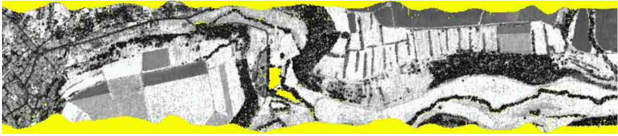
Figure 2 – Example of one (part of an) airborne laser scanning strip showing the recorded intensity values. Data courtesy of EuroSDR.
