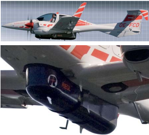
Figure 3: ALS system based on two RIEGL LMS-Q560 and Diamond Airborne Sensing DA42 MPP.
