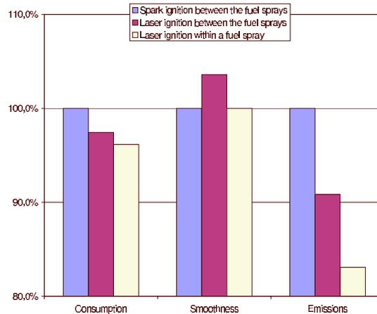
**Figure 3.** Comparison between conventional spark plug ignition and laser ignition. Laser ignition within the fuel spray of an injector shows the best results in reducing fuel consumption and exhaust emission at the same engine smoothness.
