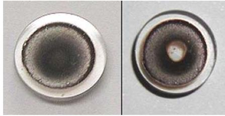
**Figure 4.** Beam entrance window: left side after 20 h operation with spark plug ignition, right side: immediately after 100 laser pulses. Beam area is cleaned by the laser beam.
