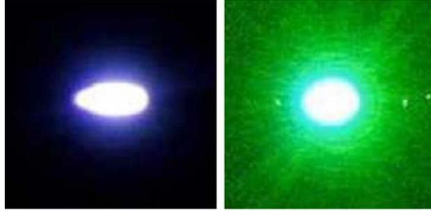
**Figure 1.** Optical breakdown in air generated by a Nd:YAG laser. Left: at a wavelength of 1064 nm, right: at 532 nm
