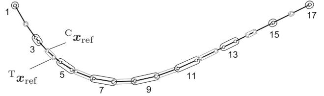
Fig. 5. Example for the variation of the step size during detected side-slip or tangential slip and corresponding interpolation of the pre-planned trajectory
