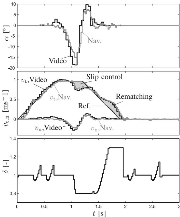
Fig. 6. Tangential and lateral velocity and side slip angle estimate and slip control during tracking of a corner, Ref. indicates the velocities associated with the reference trajectory
