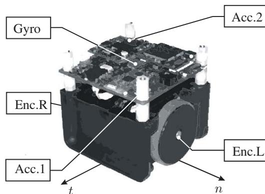
Fig. 1. Autonomous mini-robot Tinyphoon, <http://www.tinyphoon.com>
