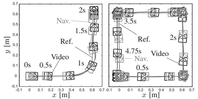
Fig. 8. Posture estimates during tracking of a corner (left) and a square (right)
