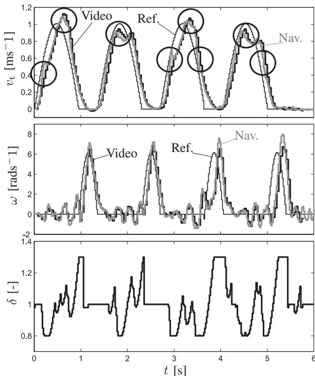
Fig. 7. Tangential velocity and yaw rate estimation and slip control during tracking of a square, Ref. indicates the velocities associated with the reference trajectory
