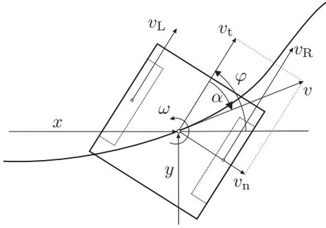
Fig. 2. Kinematics of a two-wheeled mobile robot under consideration of side-slip
