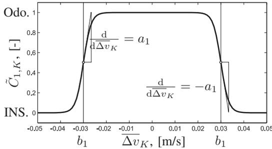
Fig. 4. Double-sided logsig-function as switch between odometric (Odo.) and inertial (INS.) navigation
