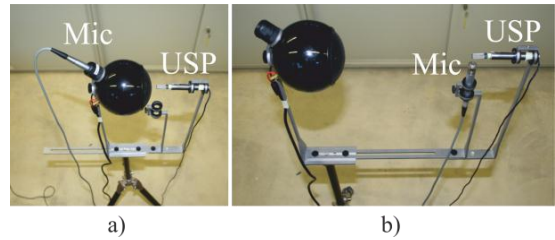
Fig. 3. Piston on a sphere: a) low frequency and b) high frequency calibration setup.
