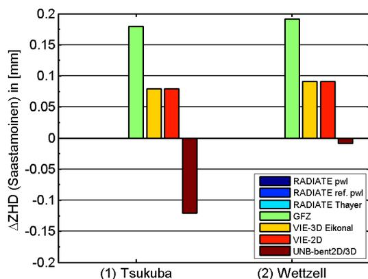
**Fig. 2** Differences in zenith hydrostatic delay determined from the equation by Saastamoinen (1972), [5] [ZHD (Saastamoinen) from a specific ray tracer minus ZHD (Saastamoinen) from RADIATE pwl]. The reference ZHD (Saastamoinen) taken from RADIATE pwl has the following absolute values: (1) Tsukuba: 2.2948 m, (2) Wettzell: 2.1662 m. Please refer to the Web version of the Proceedings to see the original color-coded version of this figure.
