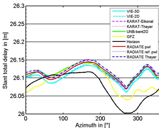
**Fig. 4** Slant total delays (STD) calculated from the total mapping factors (TMF) of different ray-tracers for Tsukuba (Tsukub32) at 5° elevation for 12 August 2008, 0 UTC. The STD is calculated with the TMF of the different ray-tracers and the zenith total delay (ZTD) of RADIATE pwl (2.5716 m). Please refer to the Web version of the Proceedings to see the original color-coded version of this figure.
