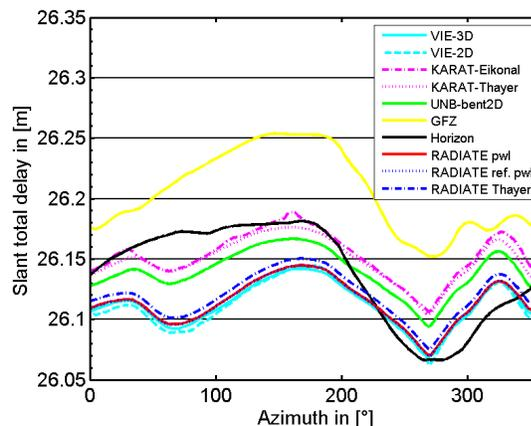
**Fig. 3** Slant total delays calculated by different ray-tracers for Tsukuba (Tsukub32) at 5° elevation for 12 August 2008, 0 UTC. Please refer to the Web version of the Proceedings to see the original color-coded version of this figure.
