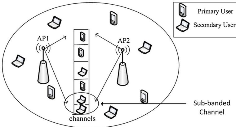
**Fig. 1** General model of spectrum sharing with channel sub-banding
