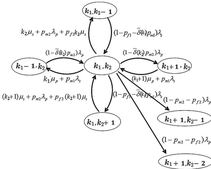
**Fig. 2** Transition diagram for channel sub-banding with unreliable spectrum sensing
