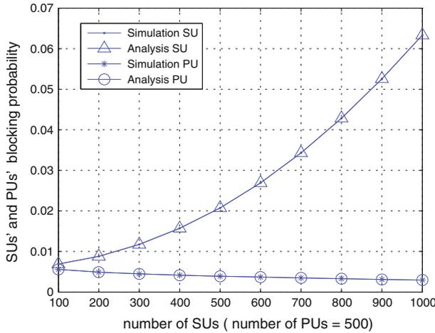
Fig. 3 Validation of PUs' and SUs' call blocking probabilities  $p_f = p_m = 0.05$
