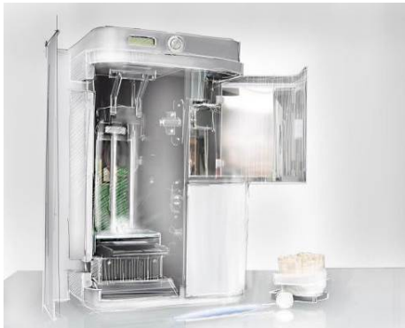
Figure 9. On the space base, the restoration and the positioning guide are manufactured using a 3D printer (image credit: space-craft Architektur, D. Krljes)
