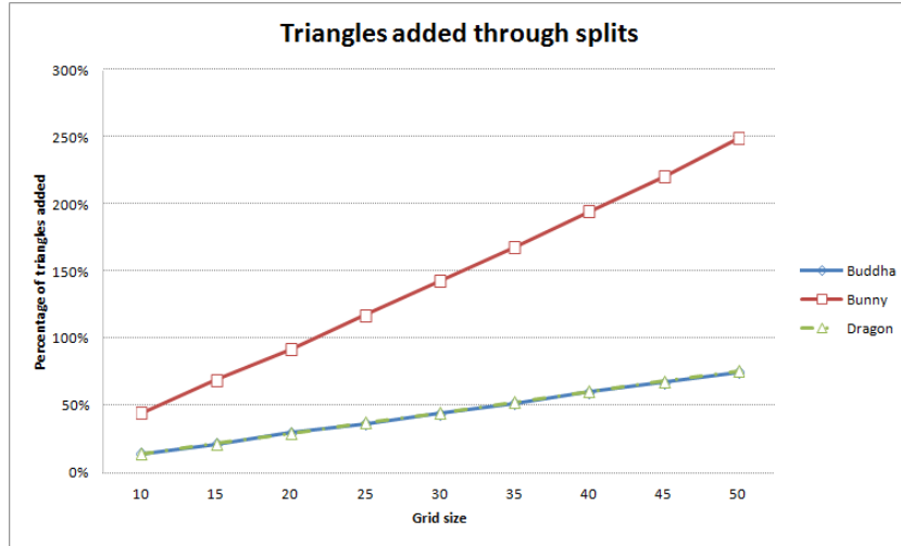
Figure 6.4: Here we can see the relative amount of triangles generated through splits for different grid sizes. The displayed linear growth suggests that increasing number of cells translate into more triangle splits and thus not reducing the overall problem size anymore.
