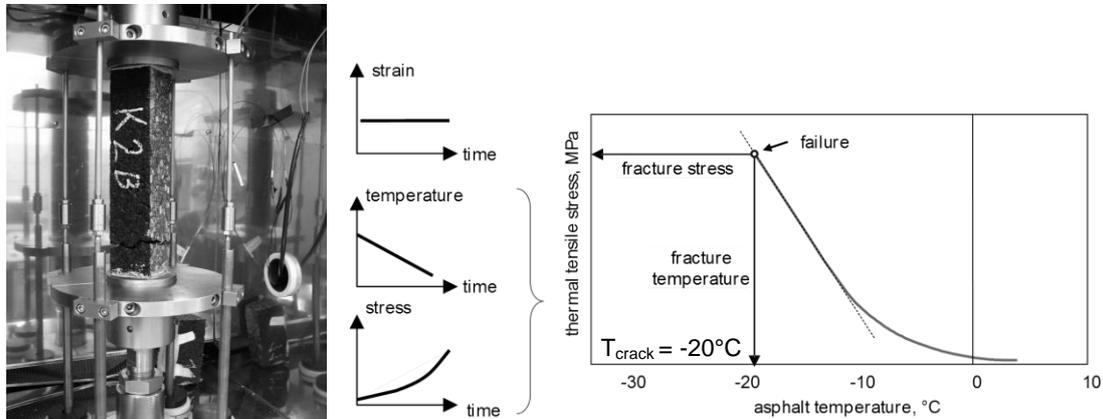
**Figure 1. TSRST: experimental setup and illustration of result (Blab & Eberhardsteiner 2009)**
