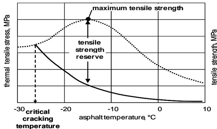
**Figure 2. Superposition of TSRST and UTST results to derive tensile strength reserve (Blab & Eberhardsteiner 2009)**
