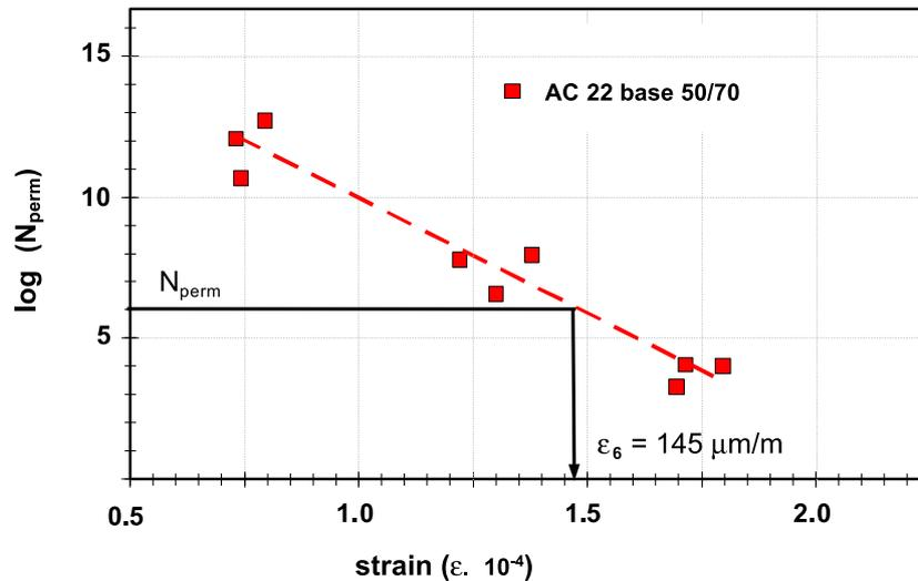
**Figure 7. Calculation of the fatigue parameter  $\epsilon_6$  for HMA type AC 22 from a strain controlled 4PBBT**
