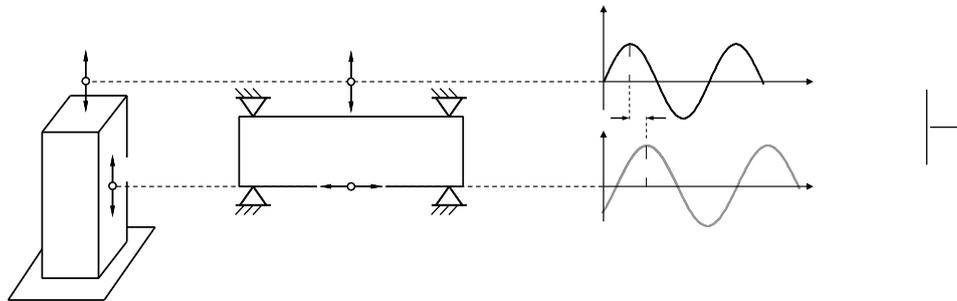
**Figure 3. Stiffness modulus ( $E^*$ ) and phase angle ( $\phi$ ) (Blab & Eberhardsteiner 2009)**
