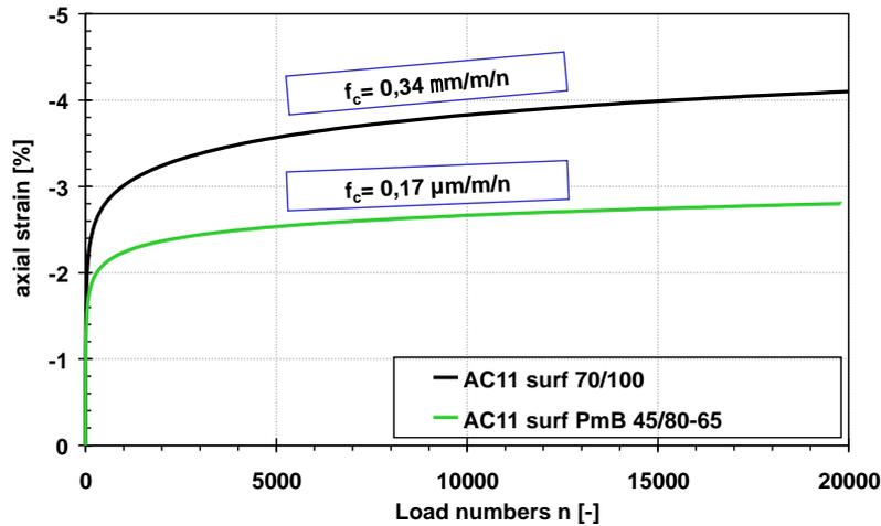
**Figure 10. Creep curves for HMA type AC 11 surface with two different of binders**
