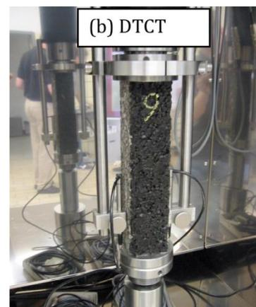
**Figure 4. 4PBBT & DTCT equipment used for stiffness and fatigue testing (Blab & Eberhardsteiner 2009)**
