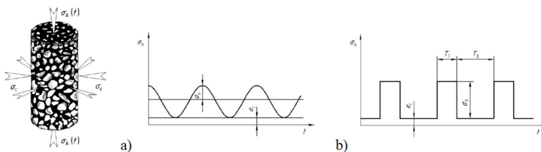
**Figure 8. a) sinusoidal shaped axial loading and b) block-impulses as axial loading, both with constant confining pressure (EN 12697-25, 2008)**
