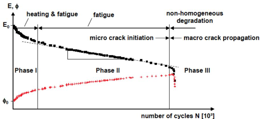
**Figure 6. Phases of AC 22 fatigue curve from a strain controlled 4PBBT (acc. to: Di Benedetto et al. 2001).**
