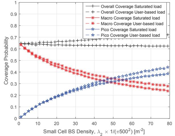
Fig. 4: Effects of small cell density on coverage probability of network.
