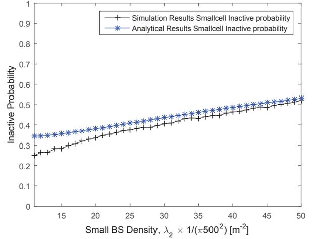
Fig. 2: Small cell inactive probability under different small cell density.
