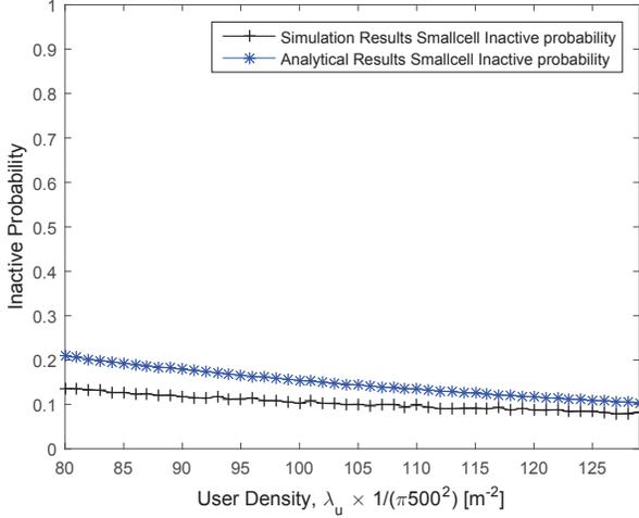
Fig. 1: Small cell inactive probability under different user density.
