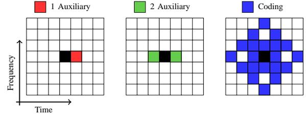
Fig. 2. In order to straightforwardly apply pilot symbol aided channel estimation in FBMC, we have to cancel the imaginary interference at the pilot positions. One auxiliary symbol wastes too much energy, two auxiliary symbols causes a further loss of data symbols and coding requires a higher computational complexity.
