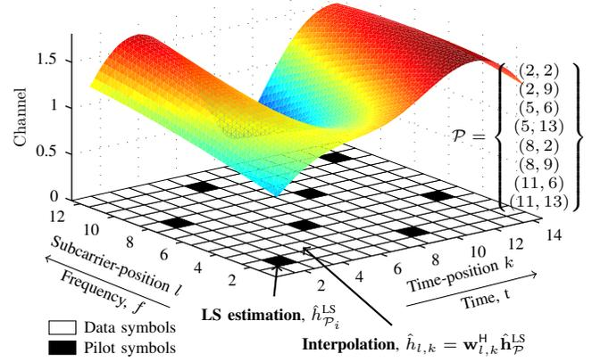
Fig. 1. Pilot-symbol aided channel estimation consists of two basic steps: Firstly, a LS channel estimation at the pilot positions. Secondly, interpolation of those LS estimates to obtain channel estimates at the data positions.
