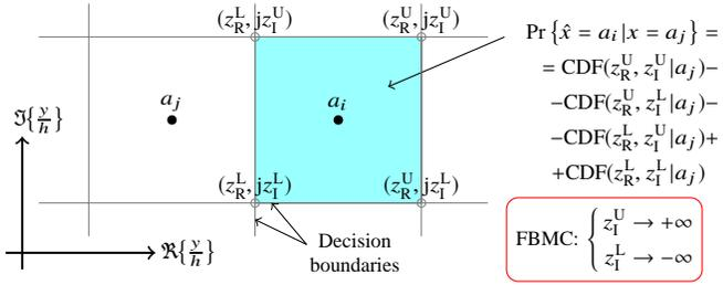
Fig. 1. For a given symbol alphabet  $\mathcal{A}$ , we apply Lemma 1 and (11)-(14) to calculate the probability that  $\hat{x}_{l,k} = a_i$  is detected, conditioned that  $x_{l,k} = a_j$  was sent, allowing us to calculate the BEP in (15).
