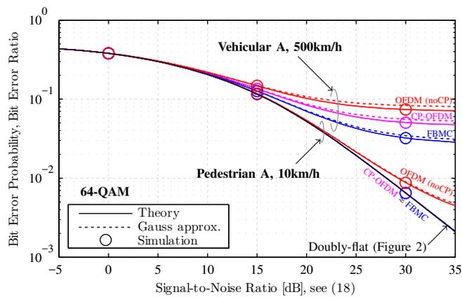
Fig. 3. Simulations validate our BEP calculations of Section III. The interference is not Gaussian distributed, so that the Gaussian approximation only provides a rough estimate of the true BEP.
