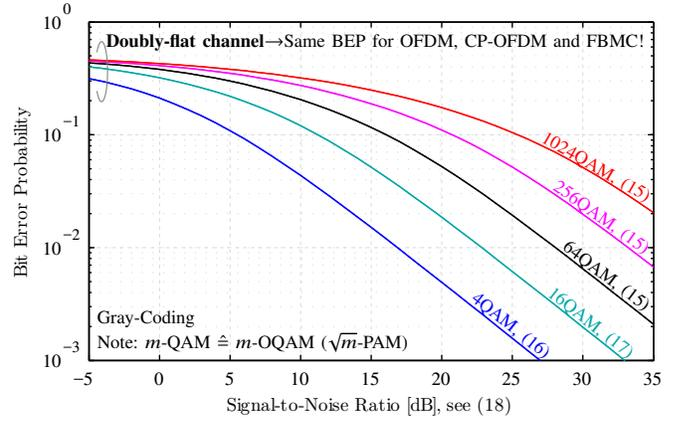
Fig. 2. Doubly-flat fading represents an important special case because it also describes the BEP for a doubly-selective channel as long as the SNR is smaller than a certain threshold, see Figure 3.
