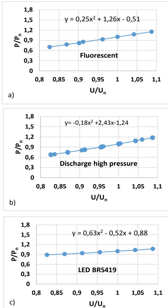
Figure 2. Active power of load versus applied voltage for different lamp types: a) fluorescent; b) discharge high pressure; and c) LED BRS419. Preferred analytical function and smoothed data curve.
