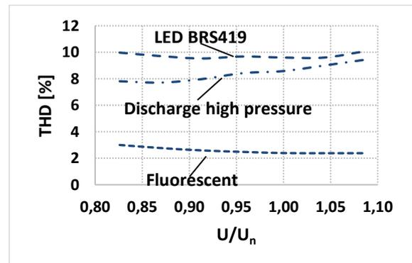
Figure 5. THD according to IEEE 1035 as a function of voltage for different lamp types.
