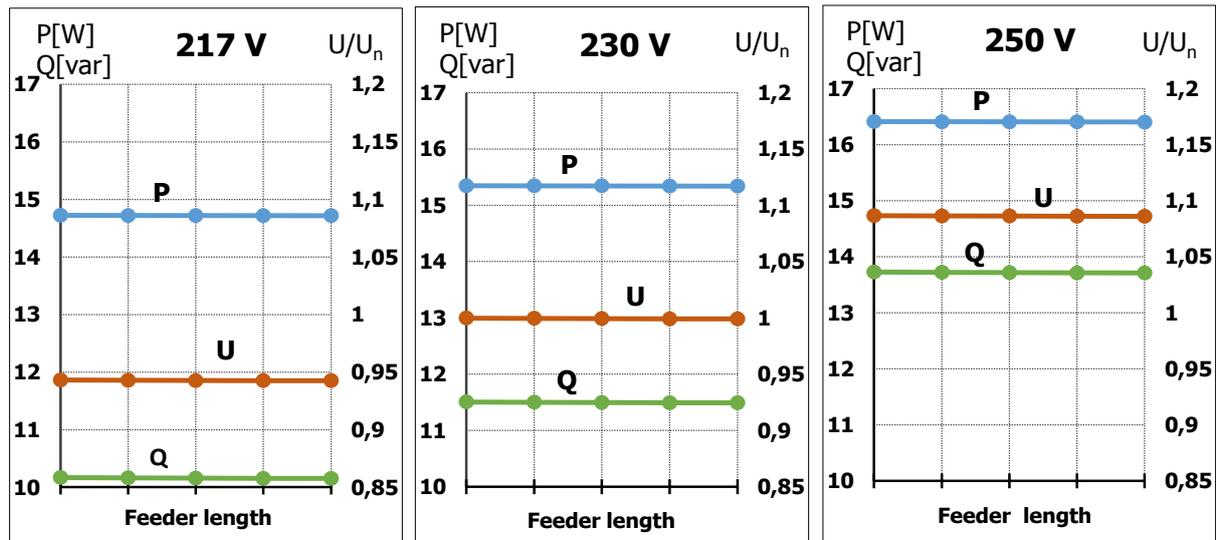
Figure 8. Active-, reactive power lamp consumption and voltage over the length of a feeder for LED lamps BRS419, for different voltage values at feeder head: a) 207V; b) 230V and c) 250V.
