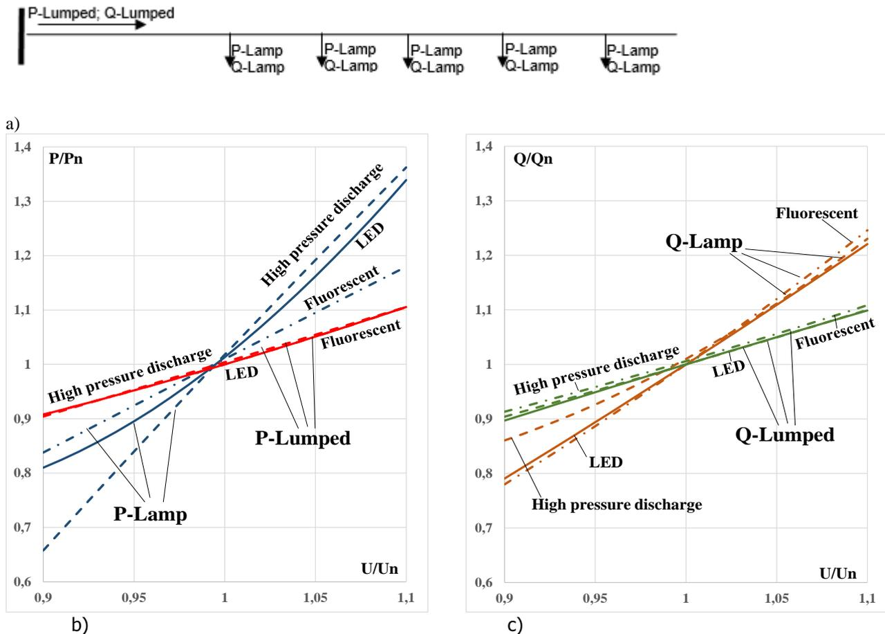
Figure 7. Power components of the static load characteristic for the individual lamp loads and lumped load at feeder head for different lamp types: a) Lighting feeder; b) active power; c) reactive power.
