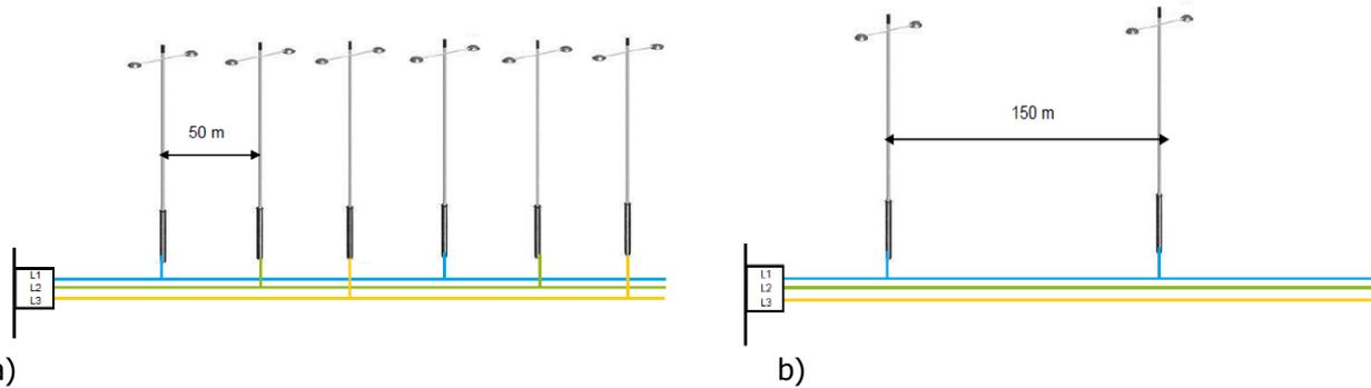
Figure 6. Overview of the connection of street lighting: a) on a three phase feeder and b) on a specific phase.
