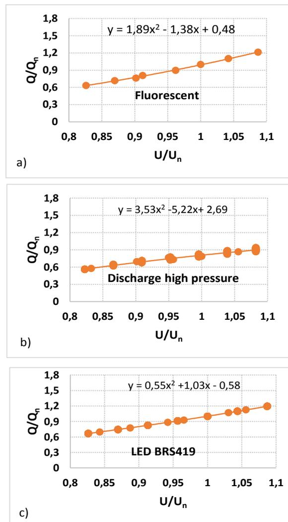
Figure 3. Reactive power of load versus applied voltage for different lamp types: a) fluorescent; b) discharge high pressure; and c) LED BRS419. Preferred analytical function and smoothed data curve.
