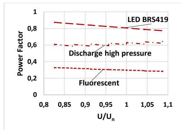
Figure 4. Power factor as a function of voltage for different lamp types.
