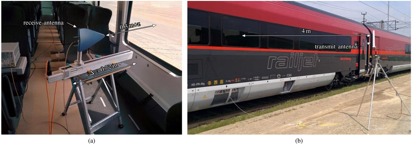
Fig. 2. Measurement setup: (a) The receive antenna inside the train is moved along the connecting line to the transmit antenna using a linear guide. (b) The transmitter is located outside the train.
