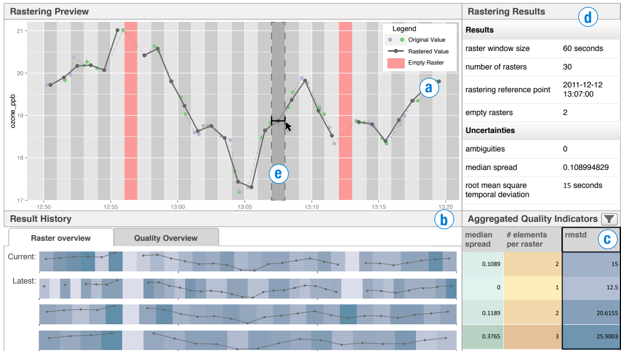
Figure 1: An overview of our interactive time series rastering approach. (a) The interactive rastering preview allows defining the raster window size through drag&drop interaction as well as comparing the current raster configuration to the original data. Alternating consecutive raster backgrounds and original value point colors per raster facilitates distinction. Empty raster intervals are highlighted by red segments. (b) In the result history view users can compare previous rastering results represented by small multiple line charts. Selecting a quality indicator (in c) overlays the small multiples with a heatmap of individual quality measures per raster. This view can be switched to the quality overview which gives multivariate quality and uncertainty information on recent raster configurations (cf. Fig. 2). (c) The aggregated quality and uncertainty indicator view features a sortable and customizable heatmap view representing the aggregated quality and uncertainty measures for each raster configuration in the history view. Color intensity corresponds to higher values (cf. Fig. 2). (d) Overview information of rastering results, including meta information, general uncertainty measures, and introduced quality issues based on calculated quality metrics. (e) Drag&Drop interactive selection of rastering window length.
